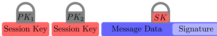
Figure 2: The makeup of a PGP message with two recipients with public keys PK_1 and PK_2 . The session key SK is separately encrypted with the two public keys, and the message data is symmetrically encrypted with the session key. The signature is optional.
